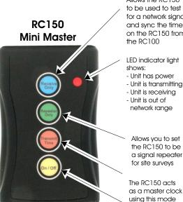
Allows the RC150 to be used to test for a network signal and sync the time on the RC150 from
